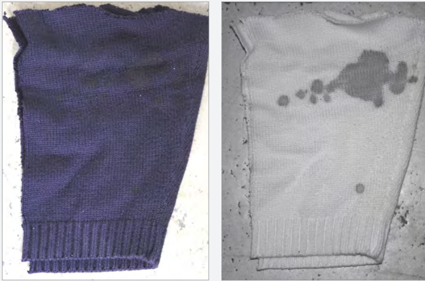
Bloodstains on wool, standard light, optimized Near Infrared Copyright Dr. M. Schulz, Institute of Legal Medicine LMU Munich
